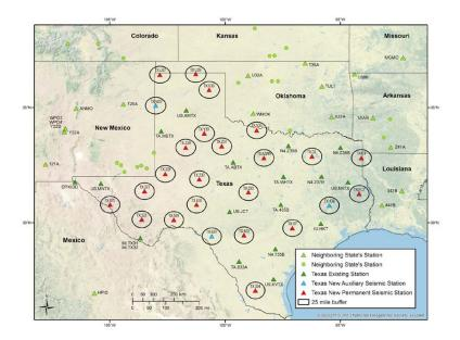
TexNet plans to install at least 22 new permanent and an additional 36 portable stations evenly spaced across Texas. *Image courtesy of the Bureau of Economic Geology.*
